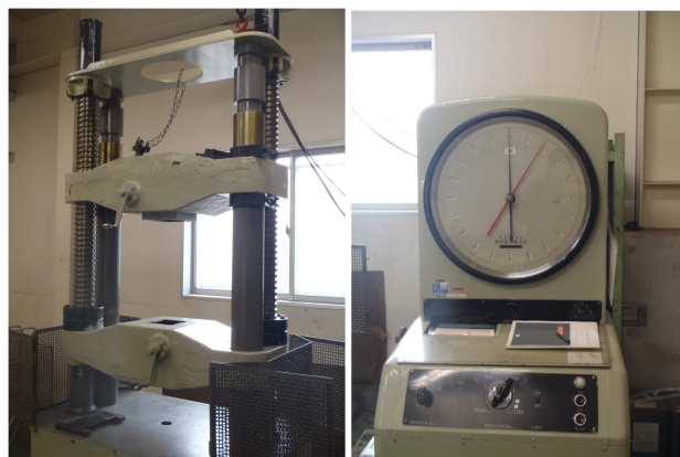
Fig. 1 Appearance of Amsler type tensile tester manufactured by Tokyo Koki Co. Ltd owned by Ishii Iron Works Co., Ltd.
