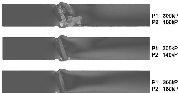
Fig.1 View of the Analysis Results with Cavitation
