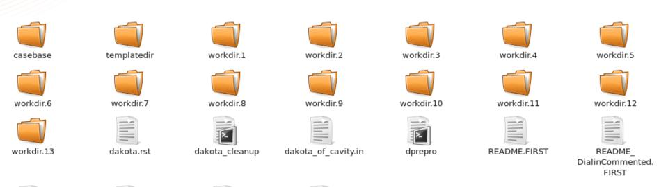
It has: copy the openFOAM case from casebase dir, create workdir\*, and launched the analysis for each of those directories with the specific velocity inlet within the range specified in the dakota\_of\_cavity.in file.
