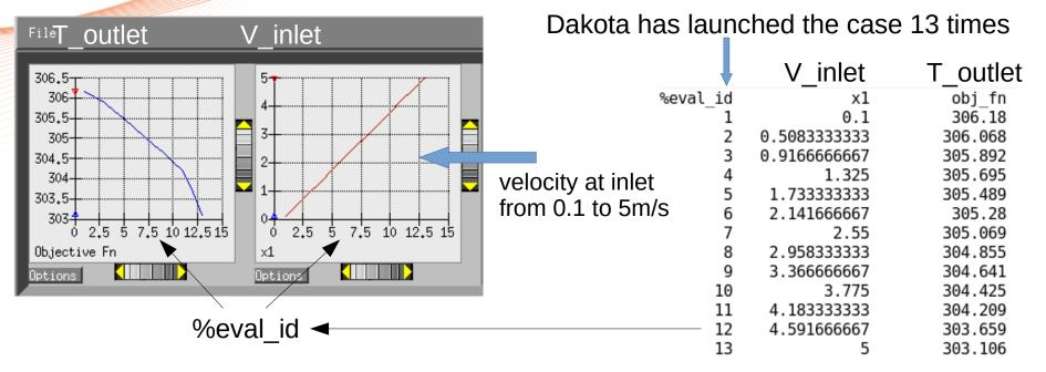
And we get as output the objective function (temperature average at the outlet).
